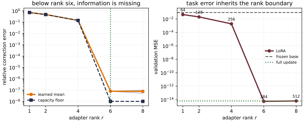
Figure 17.4.: LoRA’s rank is a real capacity constraint in a problem constructed to expose it. Five factor initializations converge to the same rank-limited relative update errors (left), closely tracking the analytic best floors from the planted diagonal magnitudes. Validation error (right) falls sharply but remains nonzero below the planted rank six; rank six, rank eight, and the unrestricted full update reach numerical zero. Counts label trainable adapter values in this deliberately small layer.
